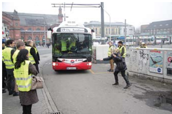
Electric bus with overhead wire charging (Siemens/Rampini-Bus from Vienna), borrowed by Bremen for a touristic route in December 2013.
