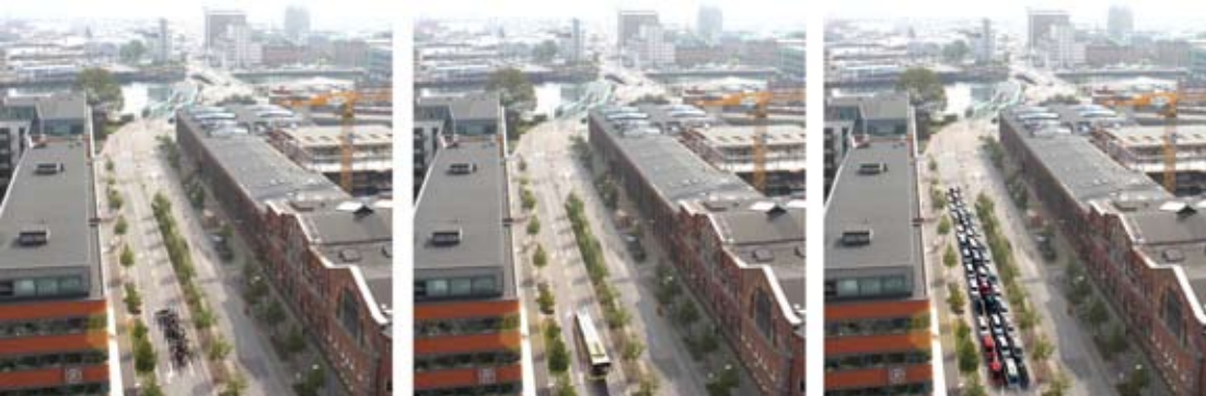
A comparison of the space required to transport the same amount of people via three different types of transportation: Cars, buses and bicycles.
