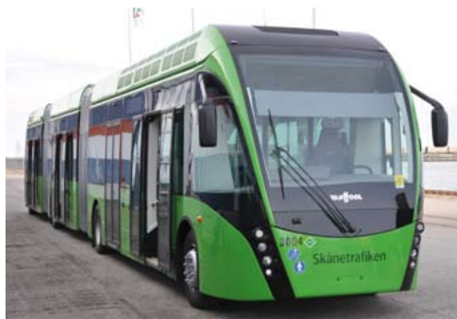
The Malmö Express is a 24 meter long gas- and electric hybrid bus and is twice the size of a normal city bus in Malmö.
